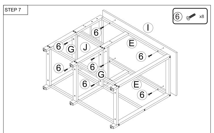
When installing the cover plate, it is recommended to first insert all corresponding screws into the corresponding holes (do not tighten a single screw separately in this step), then insert them all together and tighten the screws one by one
