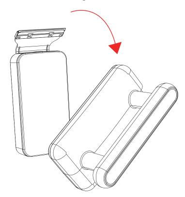
**Important reminder:** When you put both parts together outside the aquarium, always put a piece of thin cardboard between them. Because of the extremely strong magnetic force, this makes it easy to separate the two parts again later.
