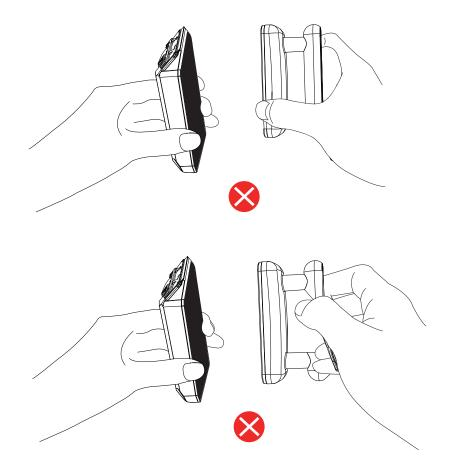
• To attach the cleaner to the aquarium glass, first hold the part with the stiff cleaning bristles against the inside of the glass and the part with the soft surface against it, offset a little. (Hold both parts firmly so that the glass is not accidentally damaged). Then carefully push both parts together slowly until the magnet grips. Then you can start with the cleaning work.
