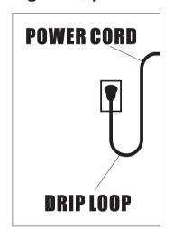
the cord and coming in contact with the receptacle. If the plug or receptacle does get wet, DO NOT unplug the cord. Disconnect the fuse to the circuit breaker that supplies power to the pump. Then unplug and examine for the presence of water in the receptacle.
