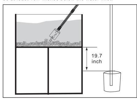
2.Immerse the water inlet into the water. Pump several times with the hand pump to draw in water. The controller can be operated with one hand and regulates the flow rate or shuts off the hose.
