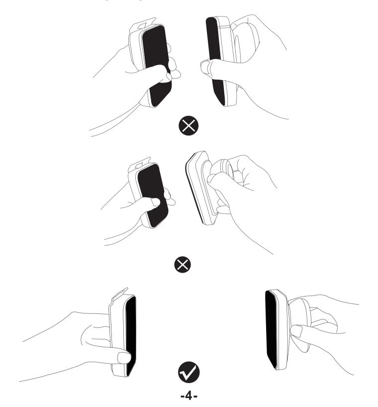
$\sqrt{\ }$  To attach the cleaner to the aquarium glass, first hold the part with the stiff cleaning bristles against the inside of the glass and the part with the soft surface against it, offset a little. (Hold both parts firmly so that the glass is not accidentally damaged). Then carefully push both parts together slowly until the magnet grips. Then you can start with the cleaning work.
