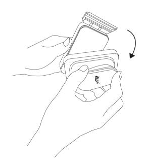
Important reminder: When you put both parts together outside the aquarium, always put a piece of thin cardboard between them. Because of the extremely strong magnetic force, this makes it easy to separate the two parts again later.
