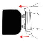
2)Pull out the clip and take off the blade from the back of the brush after use.
