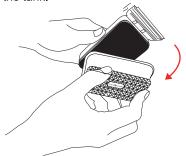
Important reminder:Do not directly stick the magnet brush and flannel brush together. Because the product has strong magnetism, it needs a strong external force to separate them when they are stuck together.
